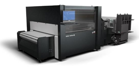
It can reach high acceleration (up to 6 g) thanks to ultralight carbon fiber bars. The extremely high dynamics, together with trajectory precision, achieved thanks to sophisticated algorithms for movement and laser control, allow unmatched productivity and quality. For laser register cutting of printed fabrics, two independent vision systems are available: the linear scanning camera which allows the cutting of printed and textured fabrics with extreme accuracy and the matrix camera.
