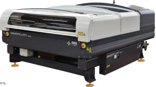
Thanks to Icaro BLU software, **Mercury** is suitable for PMMA sheets CO<sub>2</sub> cutting and marking for the vertical LED Backlight market. Mercury is also able to process several organic and composite materials, plastics, metals, fabrics, wood, paper, cardboard, corrugated, glass cork, rubber and MDF in sheet or roll.
